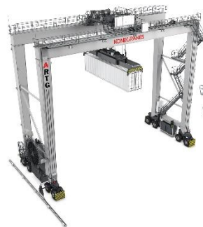
Automated RTG & RMG System (ARTG, ARMG/ASC)
