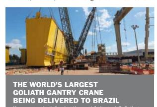
Konecranes is delivering the world's largest Goliath gantry crane to a Brazilian shipyard in Rio Grande do Sul. The crane components were delivered in autumn 2012. The crane, which will have a lifting capacity of 2,000 tons and a rail span of 210 meters, will be used for assembling Floating Production Storage and Offloading (FPSO) ships for offshore oil production projects.
